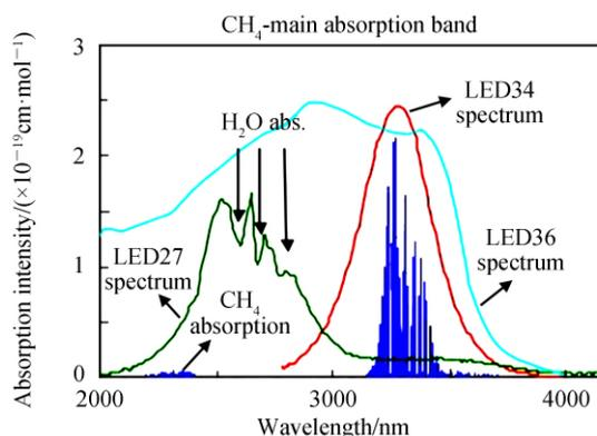
图3 LED34、LED27、PD36与CH<sub>4</sub>主吸收峰光谱关系Fig.3 Spectra of main absorption peaks of LED34, LED27, PD36 and CH<sub>4</sub>
